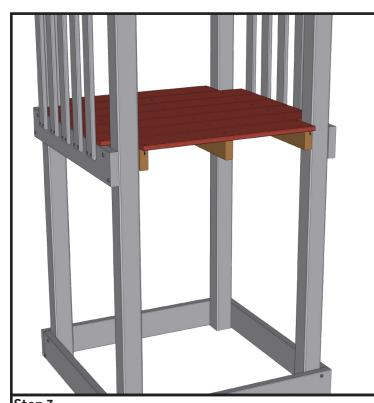
**Step 3.** Locate the floor and place it in position. The floorboards will rest on the side 2x6's to keep it in place.
