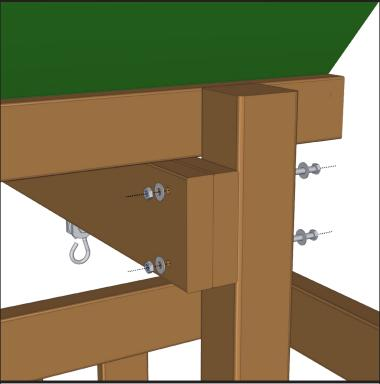
**Step 10.** Fasten the swing beam to the 4x4 post using two  $6 \frac{1}{2}$ " bolts, washer and nuts.
