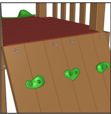
**Rock Wall** Fasten the rock wall to the tower using four 3" star head lags.
