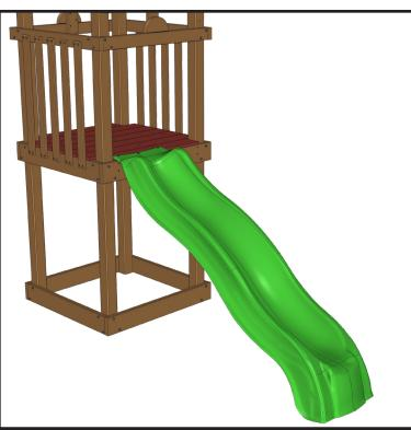
Wave Slide. Place the slide in position on the tower then fasten it with  $1 \frac{1}{2}$ " wafer head lags.
