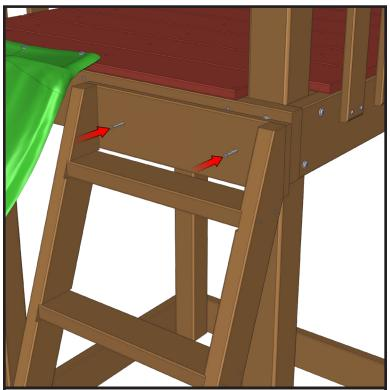
**Wood Ladder** Fasten the wood ladder to the tower using two 2" wood screws.
