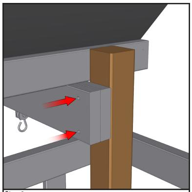
**Step 9.** Use a  $\frac{3}{8}$ " drill bit to drill through the 4x4 post using the holes in the swing beam as a guide.
