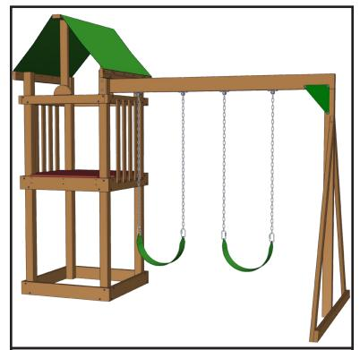
**Step 11.** Connect the swings to the swing beam at your desired height.
