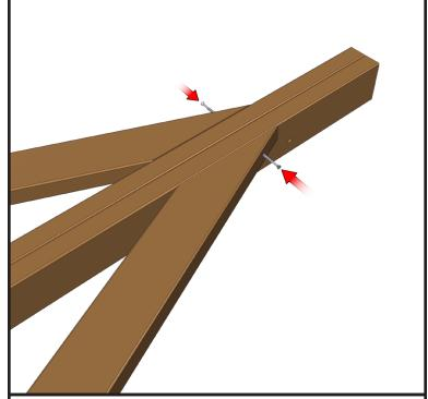
**Step 3.** Fasten the top of the 2x4 braces to the end post using 3" star head lags.
