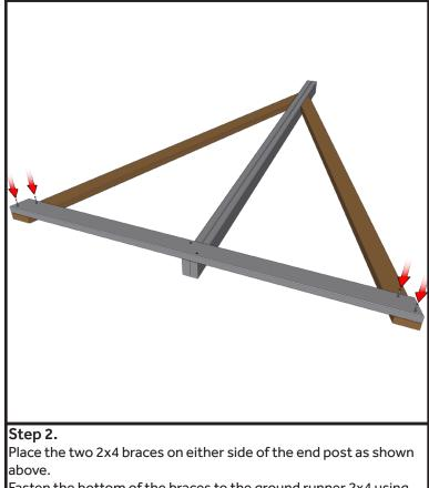
Fasten the bottom of the braces to the ground runner 2x4 using  $2\frac{1}{2}$ " wood screws.
