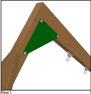
Fasten the metal support plates to the end post using the same  $3 \frac{1}{2}$  bolts.
